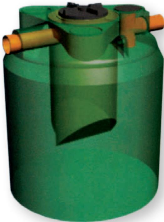
FLUXOIL de-oiler is a device for pre-treating of civil wastewaters upstream in sewage manifold. The two section of FLUXOIL have the function of separating, by floating, incoming wastewater oils and hydrocarbons and removing, by sedimentation, high specific weight materials (sand, etc.).
