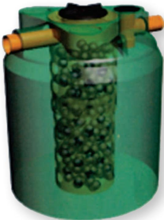
DEOXIFLUX is a trickling filter ideal for plants intended for the civil wastewater treatment that doesn't discharge into public sewer. The depuration takes place thanks to the action of anaerobic micro-organisms (that don't need any free oxygen), that originate on the surface of suitable filling bodies made by polypropylene. Trickling filters ensure effective depurating performances without energy and operating costs linked to a periodic cleaning of the system.
